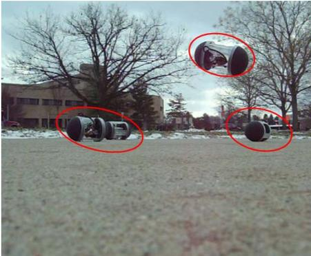
Fig. 2. Hopping sensors we designed in jumping action
